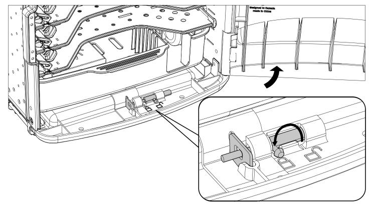
Close and lock front door of Tech Tub<sup>2</sup> to secure devices
