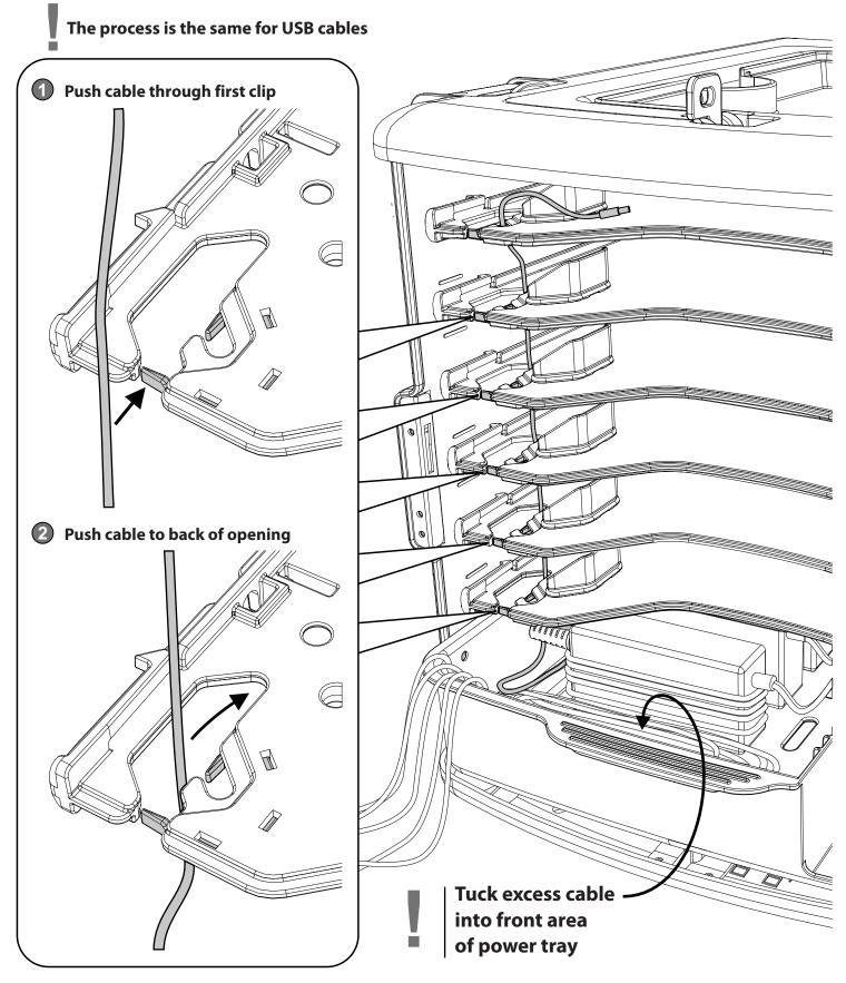
Repeat Step 13A and 13B until all remaining cables are clipped into shelves (as shown)
