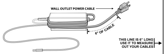
**3** Secure cables around adapter using provided hook and loop straps
