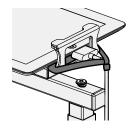
Use the provided VGA Strap to hold your VGA Adapter in place and stop it from being disconnected. (please refer to step 5)
