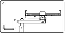
Loosen the M6 Knob to slide the Adjustment Lip into the maximum position, then tighten.
