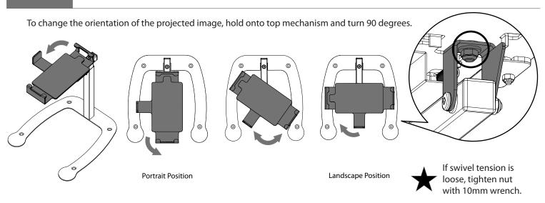
**NOTE:** Projected image may not rotate when device is rotated. To rotate image, tilt top mechanism down to allow device to adjust.
