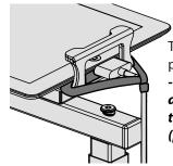
To hold the VGA cable in place use provided VGA Strap
