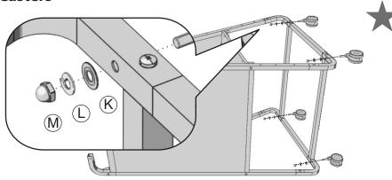
You may rest the unit on its side when installing casters
