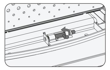
After sliding pin through bracket, lock front door of Tech Tub<sup>2<sup>\*</sup></sup> to secure devices.
